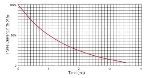
**Figure 3-4.** Current Impulse Waveform ( $I_{PP} = 8 \mu s$ )
