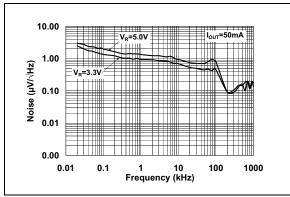
**FIGURE 2-14:** Output Noise Voltage Density vs. Frequency.
