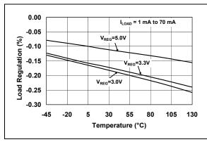
FIGURE 2-9: Load Regulation vs. Temperature.
