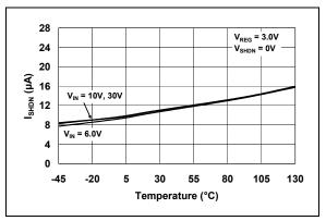
FIGURE 2-6: I<sub>SHDN</sub> vs Temperature.
