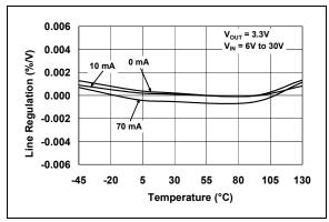
**FIGURE 2-7:** Line Regulation vs. Temperature.
