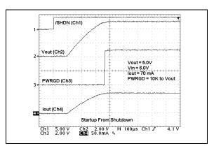
FIGURE 2-18: Startup from Shutdown (MCP1791).
