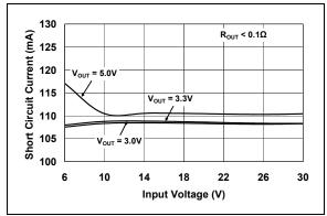
FIGURE 2-13: Short Circuit Current vs Input Voltage.
