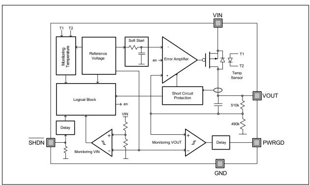
FIGURE 4-1: MCP1790/MCP1791 Block Diagram.
