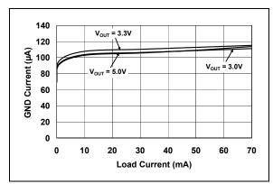
FIGURE 2-5: Ground Current vs. Load Current.
