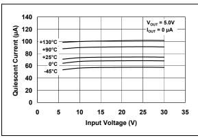
FIGURE 2-3: Quiescent Current vs. Input Voltage.
