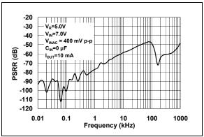
**FIGURE 2-16:** Power Supply Ripple Rejection vs. Frequency.
