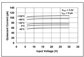
**FIGURE 2-2:** Quiescent Current vs. Input Voltage.
