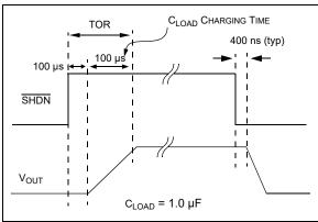
FIGURE 4-2: Shutdown Input Timing Diagram.
