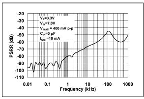
**FIGURE 2-15:** Power Supply Ripple Rejection vs. Frequency.
