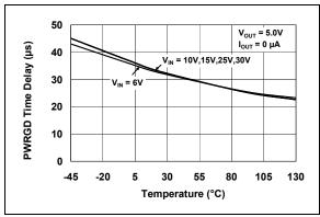
**FIGURE 2-1:** Power Good Time Delay vs. Temperature (MCP1791).
