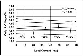
**FIGURE 2-10:** Output Voltage vs. Load Current.
