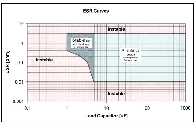
FIGURE 4-3: ESR Curves for Load Capacitor Selection.
