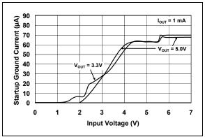
FIGURE 2-25: Startup Ground Current.
