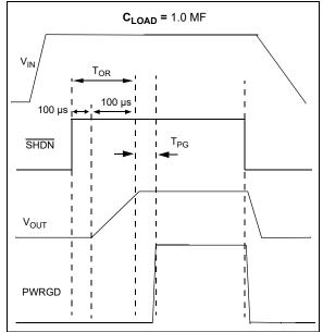
FIGURE 4-5: Power Good Timing from Shutdown.
