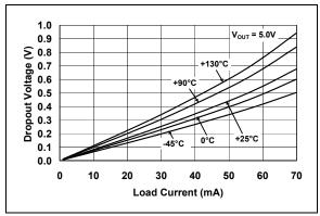
FIGURE 2-11: Dropout Voltage vs. Load Current.
