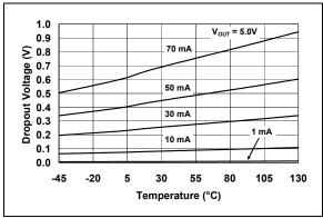
**FIGURE 2-12:** Dropout Voltage vs. Temperature.
