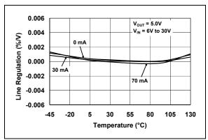
**FIGURE 2-8:** Line Regulation vs. Temperature.
