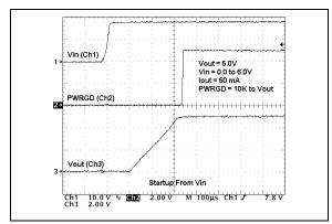
**FIGURE 2-17:** Startup from  $V_{IN}$  (MCP1791).
