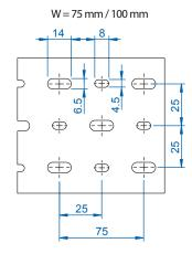
3x4, 4x4 and 6x4" duct does not have middle mounting row of slots
