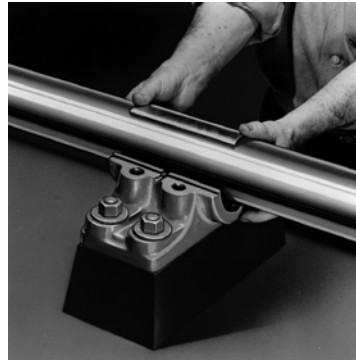
Lower half of new bushing is installed by relieving shaft pressure, prying out old bushing and rolling in new one.
