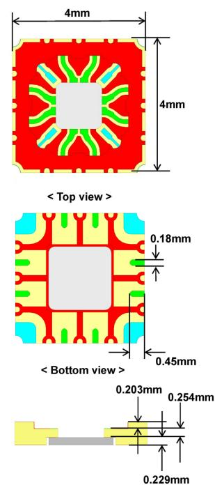
Fig. 2. CQFN 24-Pin Package Drawing (All Dimensions in mm)
