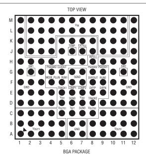
$\begin{array}{c} 144\text{-LEAD} \; (15\text{mm} \times 15\text{mm} \times 4.92\text{mm}) \\ T_{JMAX} = 125^{\circ}\text{C}, \; \theta_{JCtop} = 17^{\circ}\text{C/W}, \; \theta_{JCbottom} = 2.75^{\circ}\text{C/W}, \\ \theta_{JB} + \theta_{BA} = 11^{\circ}\text{C/W}, \; \theta_{JA} = 9.5^{\circ}\text{C/W} - 11^{\circ}\text{C/W}, \\ \theta_{BA} = \text{BOARD TO AMBIENT RESISTANCE}, \; \theta \; \text{VALUES DEFINED PER JESD 51-12} \\ & \qquad \qquad \text{WEIGHT} = 2.9g \end{array}$
