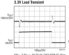
$12V_{IN},\,3.3V_{OUT},\,0A$  TO 4A LOAD STEP AT 4A/µs  $C_{OUT1},\,100\,\mu\text{F}\times\text{4}$  6.3V XSR CERAMIC 1210 CASE SIZE SWITCHING FREQUENCY 500kHz  $C_{FF}$  CAPACITOR = 47pF
