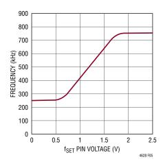
Figure 5. Operating Frequency vs f<sub>SET</sub> Pin Voltage
