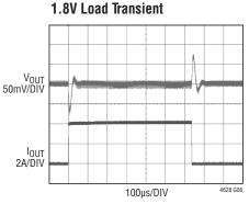
$12V_{IN}, 1.8V_{OUT}, 0A$  TO 4A LOAD STEP AT  $4A/\mu s$   $C_{OUT1}$   $100\mu F \times 4$  6.3V XSR CERAMIC 1210 CASE SIZE SWITCHING FREQUENCY 500kHz  $C_{FF}$  CAPACITOR = 47pF
