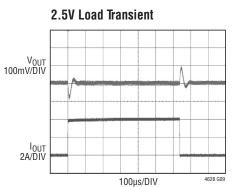
$12V_{IN}$ ,  $2.5V_{OUT}$ , 0A TO 4A LOAD STEP AT  $4A/\mu s$   $C_{OUT1}$ ,  $100\mu F$  x4 6.3V X5R CERAMIC 1210 CASE SIZE SWITCHING FREQUENCY 500kHz  $C_{FF}$  CAPACITOR =  $47\rho F$
