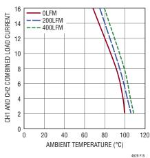
Figure 15. 24V to 1V Derating Curves, No Heat Sink
