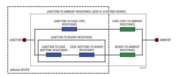
Figure 10. Graphical Representation of JESD 51-12 Thermal Coefficients
