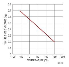
Figure 9. The 1N4148 Diode Voltage V<sub>D</sub> vs Temperature
