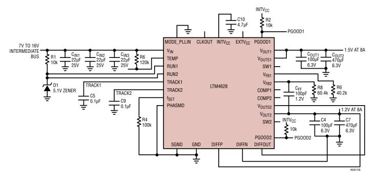
Figure 28.  $7V_{IN}$  to  $16V_{IN}$ , 1.5V and 1.2V Outputs
