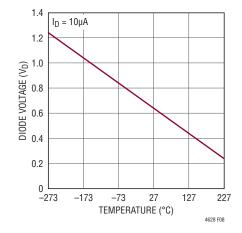
Figure 8. Silicon Diode Voltage V<sub>D</sub> vs Temperature
