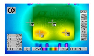
Figure 25a.12V  $_{\mbox{\footnotesize{IN}}}$  to 3.3V  $_{\mbox{\footnotesize{OUT}}},$  16A, No Heat Sink, No Airflow
