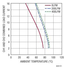
Figure 21. 24V to 3.3V Derating Curves, No Heat Sink
