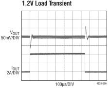
$12V_{IN},\,1.2V_{OUT},\,0$ A TO 4A LOAD STEP AT 4A/µs  $C_{OUT1},\,100\mu F$  ×4 6.3V X5R CERAMIC 1210 CASE SIZE SWITCHING FREQUENCY 500kHz CFF CAPACITOR = 47pF
