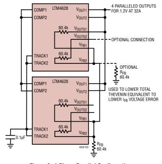
Figure 2. 4-Phase Parallel Configurations
