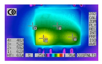
Figure 25b.12 $V_{\text{IN}}$  to 3.3 $V_{\text{OUT}}$ , 16A, No Heat Sink, 200LFM
