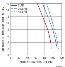
Figure 18. 24V to 1V Derating Curves with BGA Heat Sink
