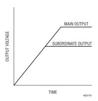
Figure 7. Output Coincident Tracking Waveform
