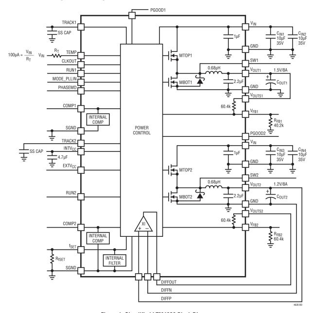
Figure 1. Simplified LTM4628 Block Diagram
