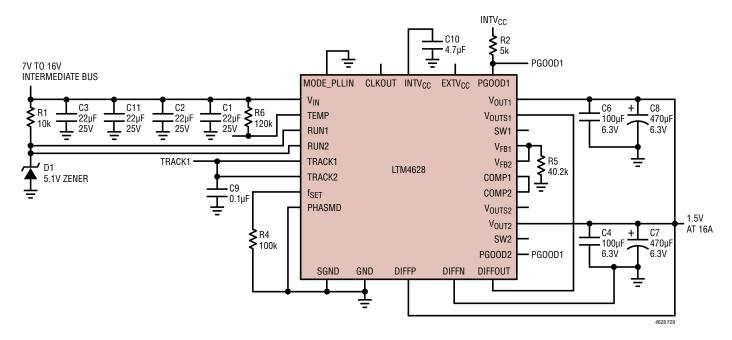
Figure 29. Two Phases, 1.5V at 16A Design
