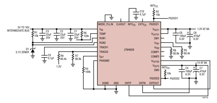
Figure 30. 1.2V and 1V Output Tracking
