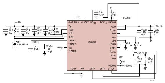
Figure 32.  $24V_{IN}$ , 5V and 3.3V Outputs
