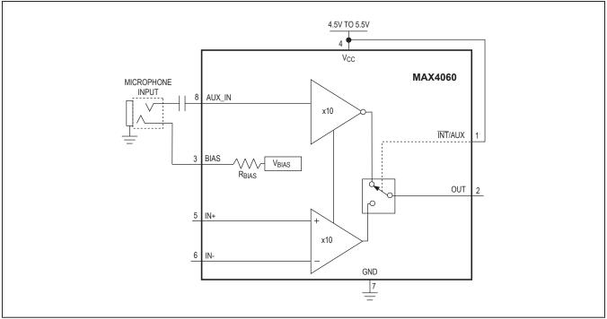
Figure 2. MAX4060 Used for Biasing a Microphone
