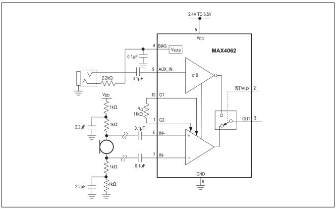
Figure 4. Remote Differential Microphone Bias Network Optimizes Noise Rejection in Long-Run, PC Board Traces
