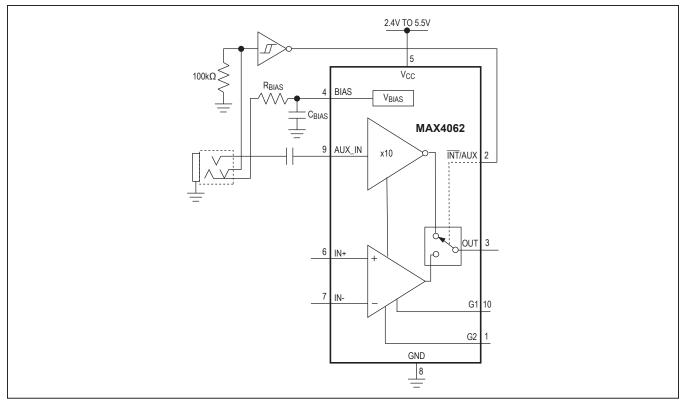
Figure 1. MAX4062 with Auxiliary Input Configuration
