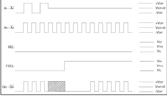
1. When the differential on the non-selected clock goes below the minimum DC differential, the outputs clock goes to an unknown state. When this happens, the FSEL pin should be asserted in order to force selection of the new input clock. The output clock will start up after a number of cycles of the newly-selected input clock.
