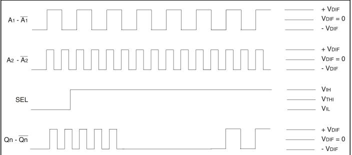
1. When SEL changes, the output clock goes LOW on the falling edge of the output clock up to three cycles later. The output then stays LOW for up to three clock cycles of the new input clock. After this, the output starts with the rising edge of the new input clock. 2. AC propagation measurements should not be taken within the first 100 cycles of startup.
