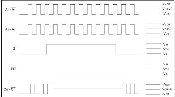
NOTE 1: It is recommended that outputs be disabled before entering power-down mode. It is also recommended that the outputs remain disabled until the device completes power-up after asserting PD.
