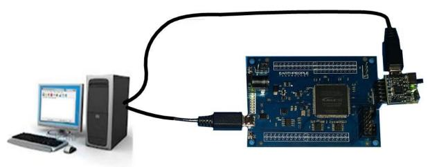
The Communications Connector provides a path between the FTDI Breakout Board and the MAX10 FPGA. It brings both the RX and TX signals into the FPGA at the following pins.
