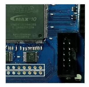
This connector uses the standard Altera Blaster connector pinout.
