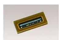
The TCD1103GFG is a high sensitive and low dark current 1500-elements linear image sensor. This device consists of sensitivity CCD chip. The TCD1103GFG has electronic shutter function (ICG). Electronic shutter function can keep always output voltage constant that vary with intensity of lights.
