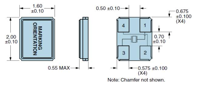
Seam Sealed Terminal Plating Thickness: Gold (0.3 to 1.0µm) over Nickel (1.27 to 8.89µm).
