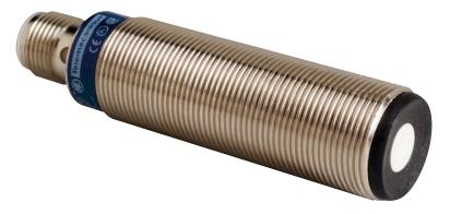
The OsiSense™ XXV18 ultrasonic sensor from Schneider Electric provides similar proximity sensing capabilities as most inductive sensors, but delivers greater sensing capabilities with respect to target color, shape or composition. These sensors are self-contained, pulse echo, ultrasonic sensing devices that both transmit and receive sonic energy in an 18 mm cylindrical housing.
