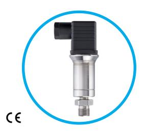
The external mount hydrostatic level transmitter, ILSEU, has a piezoresistive silicon pressure sensor which is an oil filled isolated diaphragm. The sensor and housing are made from stainless steel with a choice of internal O ring seals to ensure the product is suitable for a wide range of applications.
