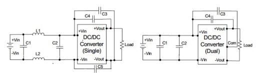
Input filter components (C1 $\sim$ C5, L1/L2) are used to help meet conducted emissions.
