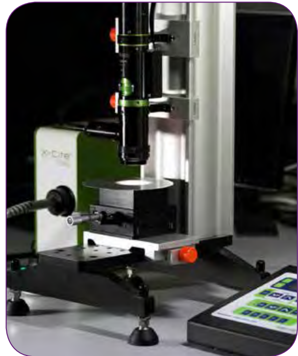
Fig. 2: Vertical X 95 construction for our micro-inspection Optem FUSION system.
