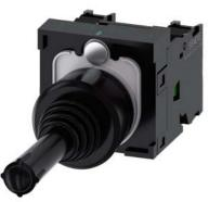
Coordinate switch, 22 mm, round, plastic, black, 2 switch positions, vertical, momentary contact type, without mechanical interlocking in O position, with holder, 1 NO, 1 NO, screw terminal, with laser labeling, upper case
