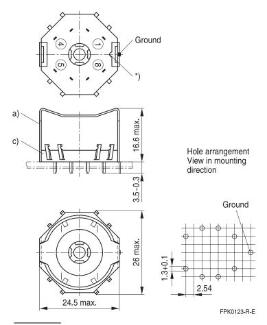
\*) This recess must be on the side of the grounding pin to ensure that the yoke locks in position.
