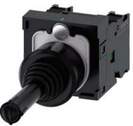
Coordinate switch, 22 mm, round, plastic, black, 2 switch positions, horizontal, momentary contact type, without mechanical interlocking in O position, with holder, 1 NO, 1 NO, screw terminal, with laser labeling, lower case
