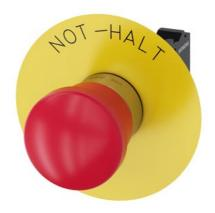
EMERGENCY STOP mushroom-type actuator, 22 mm, round, metal, shiny, red, 40 mm, positive latching, according to EN ISO 13850, pull-to-unlatch mechanism, with yellow backing plate, inscription: NOT-HALT, with holder, 1 NC, spring-type terminal, Z=20-unit packaging
