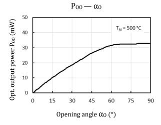
Optical output power ( $P_{00})$  versus opening angle  $\alpha_0$  (integral rotation of a cone) at 500°C  $T_{\text{M}}$
