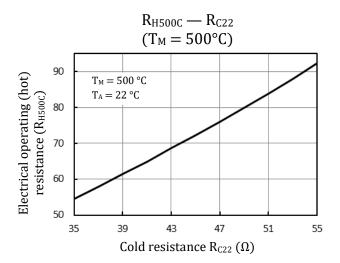
Electrical operating (hot) resistance  $R_H$  versus electrical cold resistance  $R_{C22}$  at  $T_A = 22^{\circ}C$
