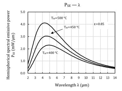
Hemispherical spectral emissive power of EMIRS200 chip surface with a typical emissivity (mean from 2 to 14  $\mu$ m) of  $\epsilon$ =0.85
