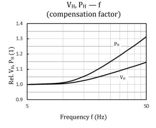
Relative (to RO) electrical drive values heater voltage  $V_{\text{H}}$  and power  $P_{\text{H}}$  versus frequency f for compensation
