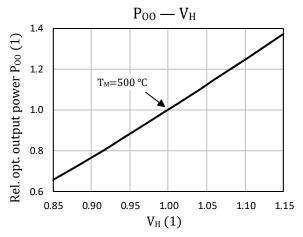
Relative change of optical output power ( $P_{00}$ ) by changing heater voltage ( $V_{\text{H}}$ )
