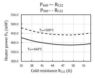
Mean  $^{1}$  and upper bound of heater power  $P_{\text{H}}$  vs. cold resistance  $RC_{22}$
