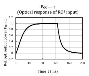
Optical response time (relative optical output power  $P_{00}$ ) of a rectangular voltage pulse (RO¹ conditions)
