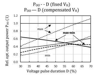
Relative (to D=62%) max, min, max-min values of optical output power ( $P_{00}$ ) versus duty cycle D with fixed and compensated  $V_{\rm H}$
