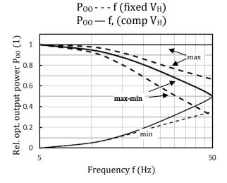
Relative (to RO) max, min, max-min values of optical output power ( $P_{00}$ ) versus frequency f with fixed and compensated  $V_{\text{H}}$
