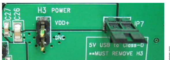
Figure 3. Connecting USB Power Supply to SSM2380
