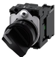
Selector switch, Illuminable 22 mm, round, plastic, black, knob, short 2 switch positions O-I, latching, 10:30h/13:30h, with holder, 1 NO, screw terminal
