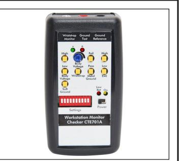
Figure 7. SCS CTE701 Workstation Monitor Checker
