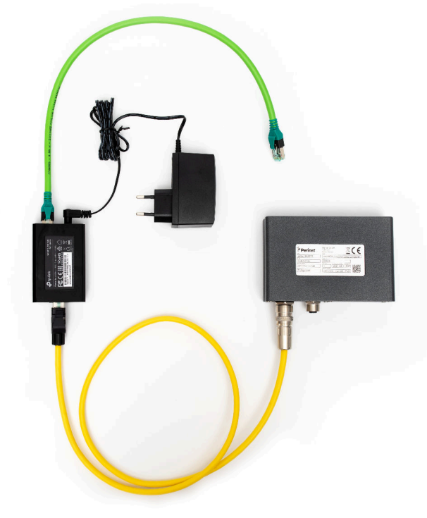
Figure 9: Connecting periMICA with PoE Injector
