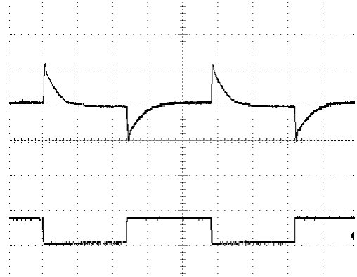
Figure 4. LTC3423 Transient Response ( V_{IN}=1.5V , I_{OUT} from 50mA to 350mA; Top Trace: V_{OUT} , 50mV/ DIV AC coupled; Bottom Trace: I_O , 500mA/ DIV)
