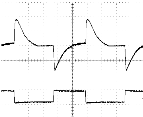
Figure 5. LTC3424 Transient Response ( V_{IN}=1.2V , I_{OUT} from 50mA to 500mA; Top Trace: V_{OUT} , 50mV/ DIV AC coupled; Bottom Trace: I_O , 500mA/ DIV)
