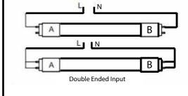
Input voltage: 120-277Vac 50/60Hz
