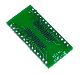
SOIC-28, SOP-28, SMD to DIP Adapter
