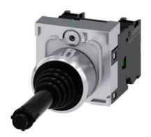
Coordinate switch, 22 mm, round, metal shiny, black, 2 switch positions, horizontal momentary contact type, with mechanical interlocking, in O position, with holder, 1 NO, 1 NO, screw terminal, Z=20-unit packaging
