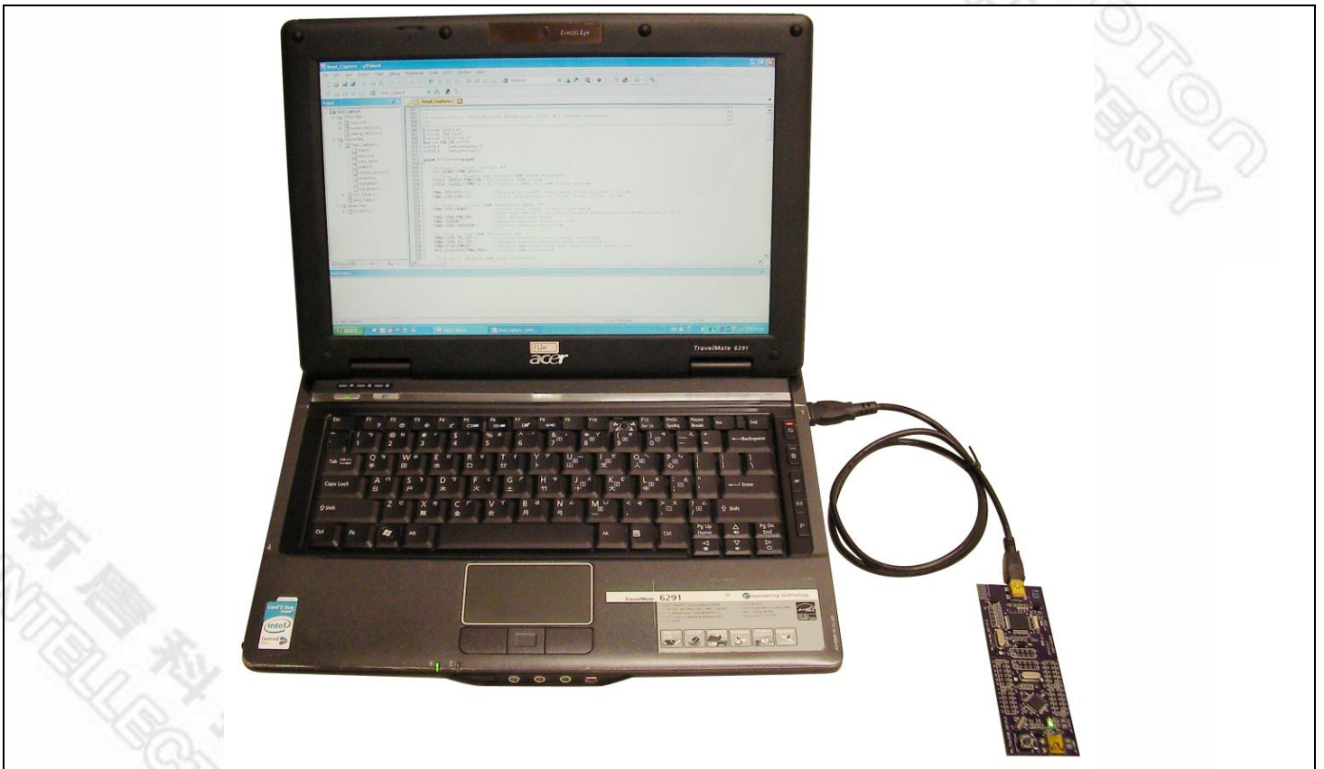
Figure 4-1 NuTiny-SDK-NUC122-64P Hardware Setup
