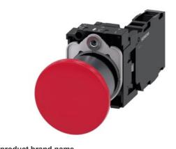
Mushroom pushbutton, 22 mm, round, plastic with metal front ring, red, 40mm, latching, pull-to-unlatch mechanism, with holder, 1 NO+1 NC, screw terminal, with laser labeling, upper case and lower case, always upper case at the beginning of the word
