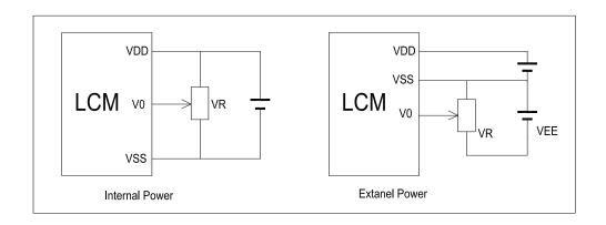
$V_{DD^{\sim}}V_0$ : LCD Driving voltage
