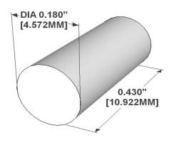
All measurements are in inches [millimeters]
