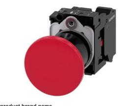
Mushroom pushbutton, 22 mm, round, plastic, red, 40mm, latching, pull-tounlatch mechanism, with holder, 1 NC, spring-type terminal, with laser labeling, upper case and lower case, always upper case at the beginning of the word
