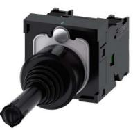
Coordinate switch, 22 mm, round, plastic, black, 2 switch positions, vertical latching, without mechanical interlocking, in O position, with holder, 1 NO, 1 NO, screw terminal, with laser labeling, lower case
