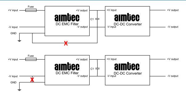
Note: Connections marked with X interfere with this filter modules performance and should therefore not be used
