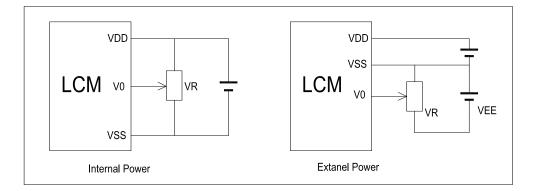
$V_{DD-V_0}$ : LCD Driving voltage VR: 10k~20k
