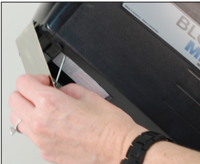
Figure 4. Releasing the filter
