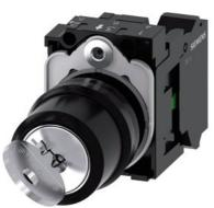
RONIS key-operated switch, 22 mm, round, plastic, lock number SB30, with 2 keys, 2 switch positions O-I, latching, 10:30h/13:30h, key removal O+I, with holder, 1 NO, spring-type terminal, possible special locks: SB31, 421, 455, with laser labeling, upper case
