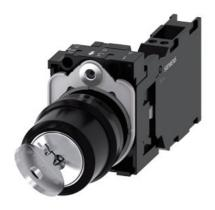
RONIS key-operated switch, 22 mm, round, plastic, lock number SB30, with 2 keys, 2 switch positions O-I, latching, 10:30h/13:30h, key removal O+I, with holder, 1 NO+1 NC, spring-type terminal, possible special locks: SB31, 421, 455, with laser labeling, upper case and lower case, always upper case at the beginning of the word
