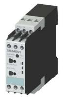
Insulation monitoring relay for ungrounded (IT) supply systems up to 400 V AC, 50-60 Hz Measuring range 1-100 kohm Supply voltage 24-240 V AC/DC 22.5 mm, 1 change-over contact screw terminal
