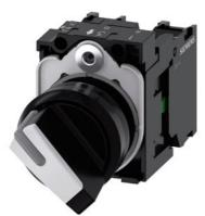
Selector switch, illuminable, 22 mm, round, plastic, white, selector switch, short, 2 switch positions O-I, latching, 10:30h/13:30h, with holder, 1 NO, 1 NC, screw terminal, with laser labeling, upper case and lower case, always upper case at beginning of line
