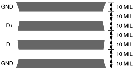
Figure 19. Arrangement of Signal Tracks
