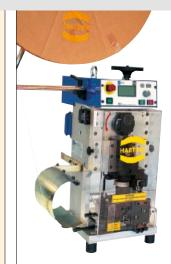
Quick change tool for D-Sub (AWG 28-24) D-Sub (AWG 24-20) D-Sub high density (AWG 26-24)
