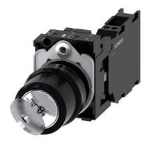
RONIS key-operated switch, 22 mm, round, plastic, lock number SB30, with 2 keys, 2 switch positions O-I, latching, 10:30h/13:30h, key removal O+I, with holder, 1 NO+1 NC, spring-type terminal, possible special locks: SB31, 421, 455
