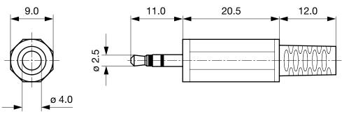
Cable diameter max. 4.0 mm
