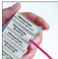
Step 3 Insert wire into marker
