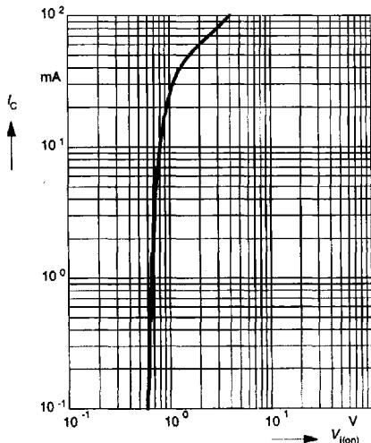
**Collector-Emitter Saturation Voltage**
