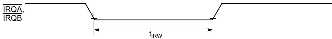
Figure 10-6 External Interrupt Timing (Negative Edge-Sensitive)
