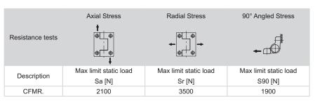
The max static load is the value above which the material may break thus prejudicing the hinge functionality. Obviously, a suitable factor, according to the importance and the safety level of the specific application must be applied to this value.
