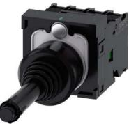
Coordinate switch, 22 mm, round, plastic, black, 4 switch positions, momentary contact type, with mechanical interlocking in O position, with holder, 1 NO, 1 NO, 1 NO, screw terminal
